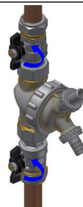
4 - Connect the pipes to the two hose connections of the connector, open the ball valves restarting the system and perform the flushing.
