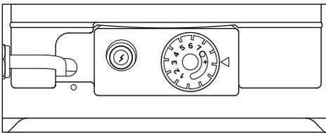
Press knob B fully in and hold it there; now press the piezoelectric igniter C. Check for a flame through hole A. Once the flame is on, continue holding knob B pressed in for a further 20 seconds or so. If the pilot flame does not stay on, repeat the above procedure.
